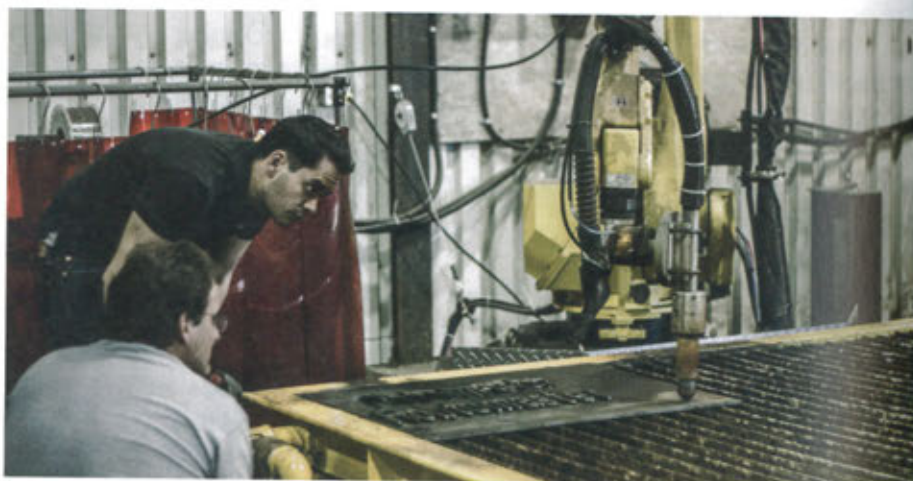
The robotic workcell for plasma cutting and welding combined with Robotmaster's robotic programming system has helped to increase production efficiencies at Groupe Gravel's operation in Mariville, QC.
